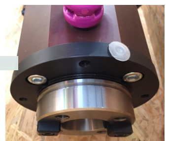
Tool spindle (ground) Integrated sealing air flange
