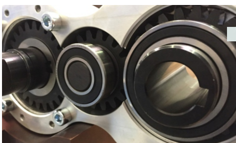
Upper Gear gears hardened and ground
