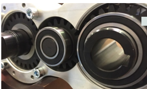
Upper Gear gears hardened and ground
